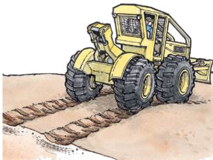
Deep compaction from the pressure and vibration of heavy equipment can decrease tree growth and cause runoff and erosion on slopes.
