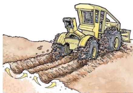
Major soil displacement is the lateral movement of soil, which often produces ruts that can change natural drainage and increase erosion.
