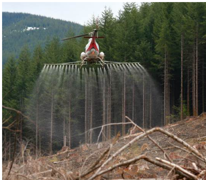
Helicopters are a cost-effective method for applying herbicides on larger forest ownerships. Drones are also becoming more common.
