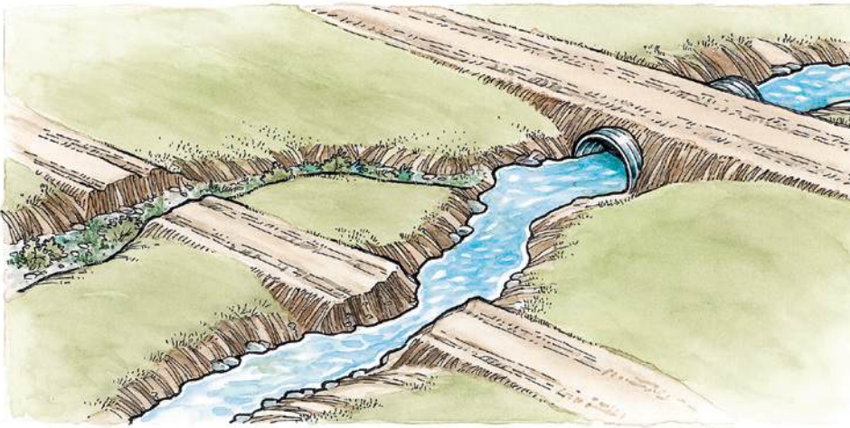
In this example, a minor relocation of the road prism results in only one culvert being reinstalled for road access. This reduces maintenance and allows the side channel below the new crossing to be restored to a more natural condition.
