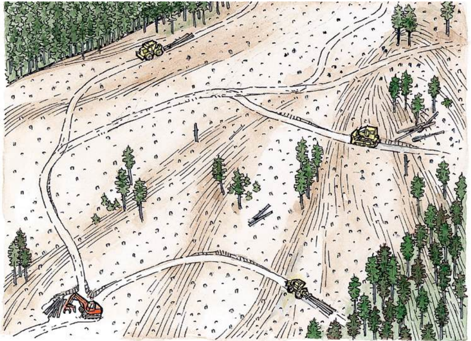
On gentle slopes, the branching skid trail pattern has one or more main trails from which other trails branch off to provide access to the area.
